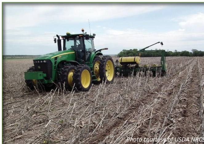
Special planting equipment limits soil disturbance
